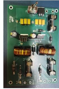
Figure 14b: Power Distribution board
