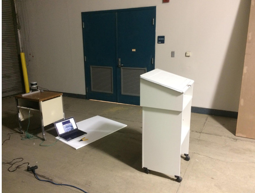
Figure 1: Test setup that we constructed for testing the LIDAR with a moving object. I rolled the lectern across the basement level while Hari and Shivang gathered data to get a gauge of how the Velodyne LIDAR performed at different distances.
