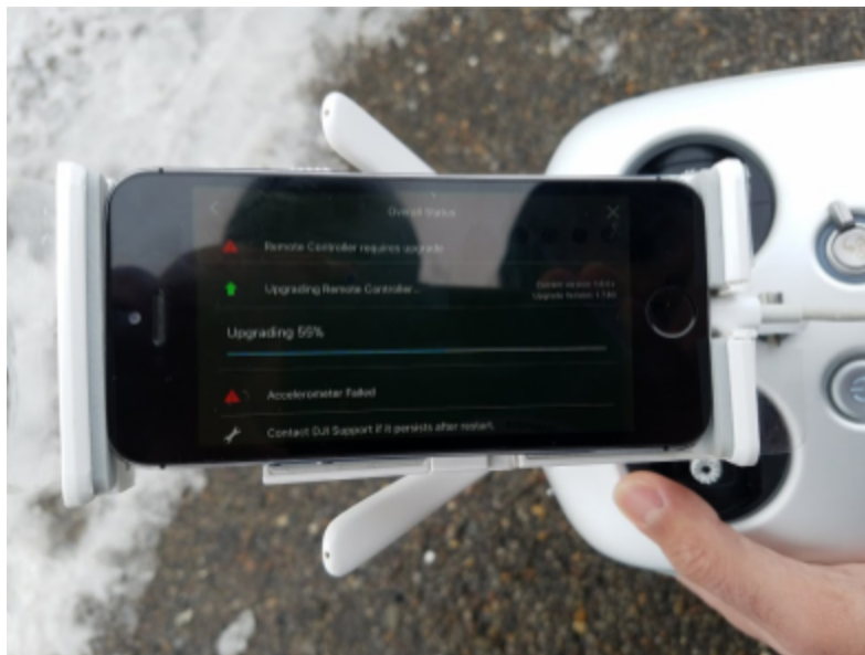
Figure 2: IMU error we experienced during the test flight
