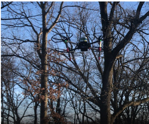
Figure 2: DJI M100 with Velodyne VLP16
