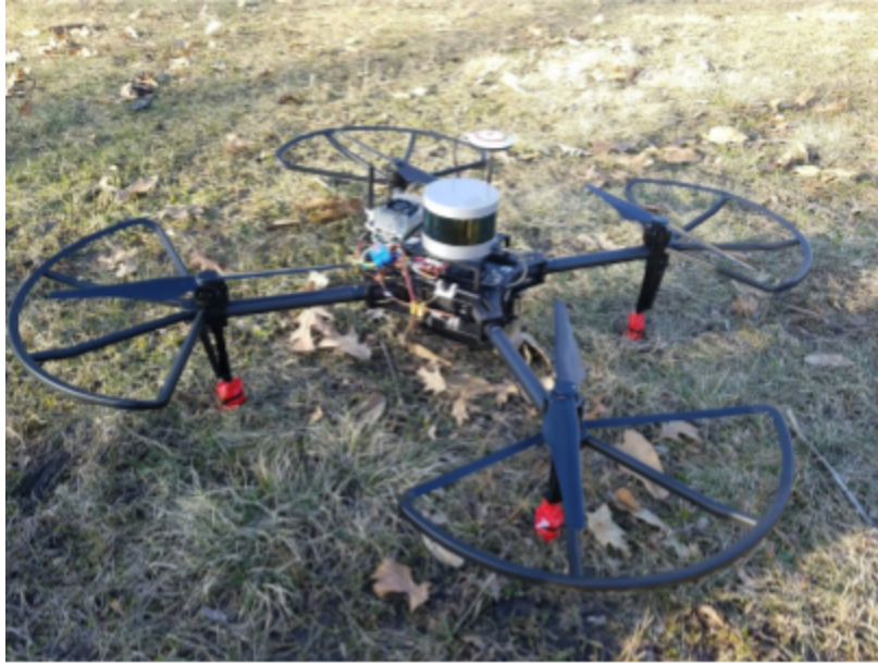
Figure 3: Flight system with LIDAR and Jetson onboard ready to detect obstacles
