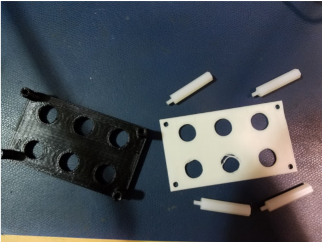
Figure 1: New Jetson mount (left) and old Jetson mount (left). The new Jetson mount holds the computer lower to prevent occlusion and incorporates spacers in the design to reduce weight and increase stiffness.
