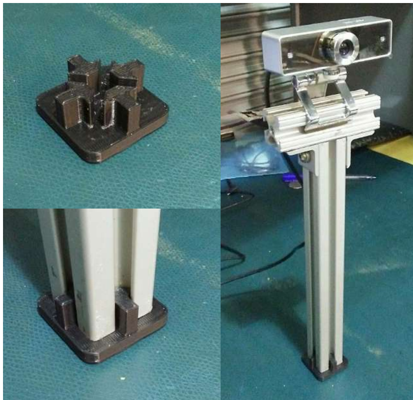
Figure 1: Top Left: 3D Printed Part, Bottom Left: Mating with vertical extrusion, Right: With the rest of skeleton + Camera
