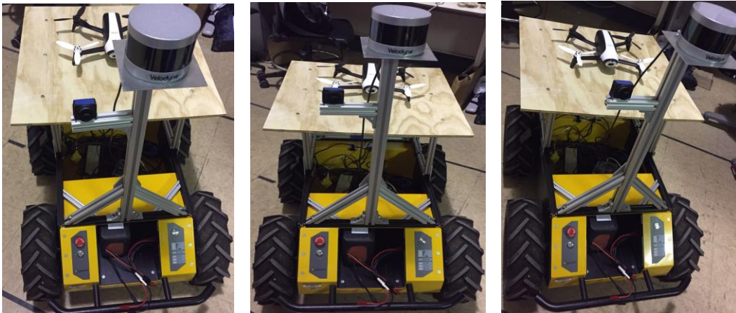
Fig.5 Mechanical mounting for Velodyne, drone and camera
