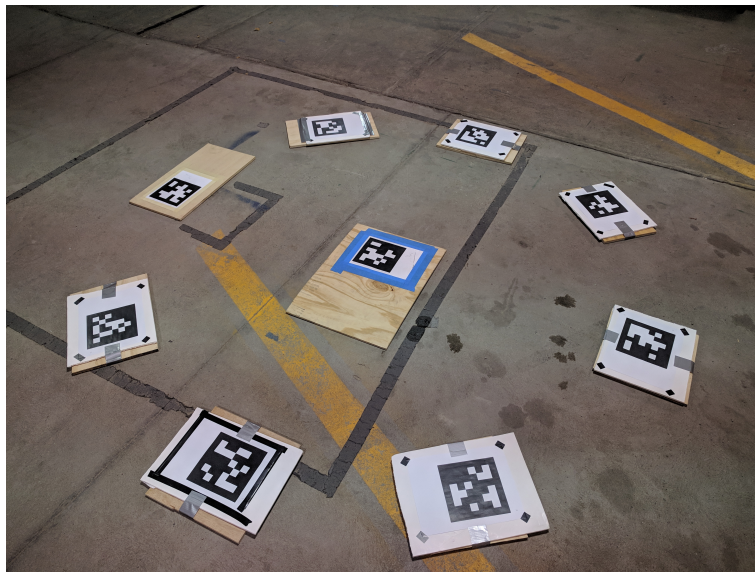
Figure 2: Picture of 8 April Tags placed in a circle of radius 1m around tag 0
