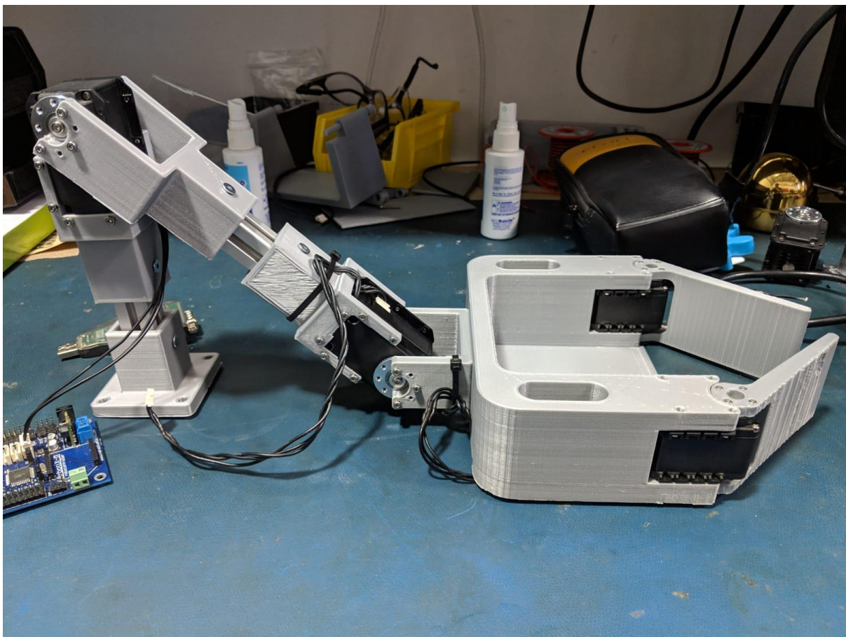
Figure 1. Manipulator with motors assembled and connected in series
