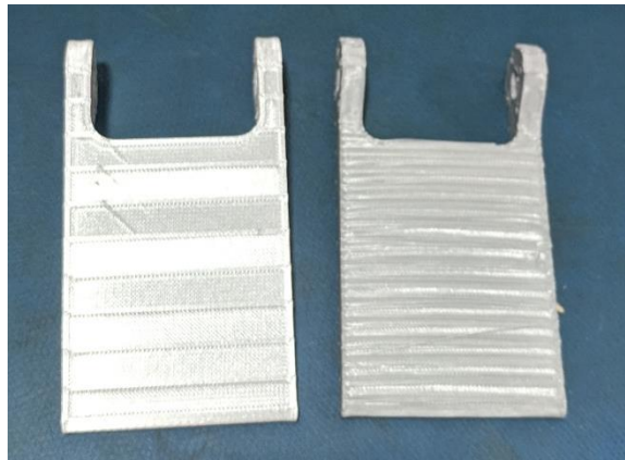
Figure 5 New paddle size with slick surface outside and coarse surface inside
