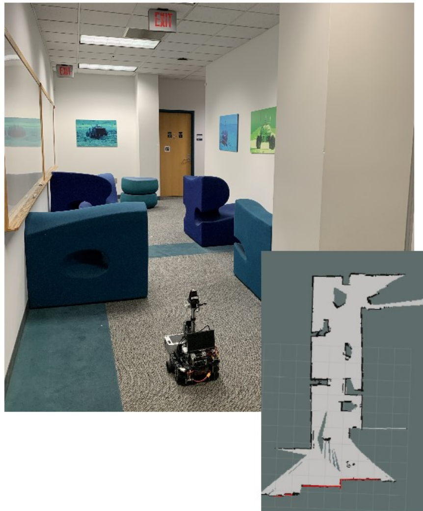
Fig 2. 2D map of the room with Hokoyu planar LiDAR
