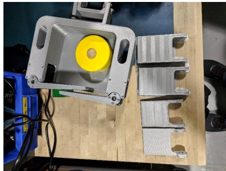
Figure 1 Paddle design options. Shown overlapping paddles for "pinball" action
