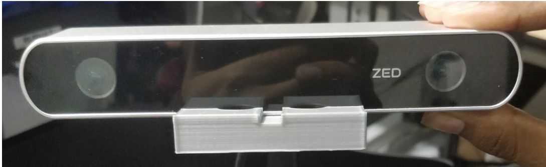
Figure 2 ZED camera fits in the 3D printed mount
