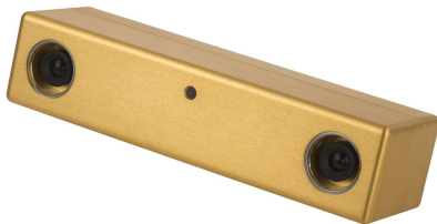
Figure 8. Bumblebee stereo camera [4]
