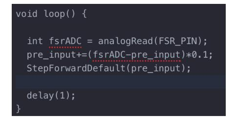
where fsrADC is the input value read from port A0. For us to achieve more stable input flow, we update only one tenth the difference between previous input and current input. Then, the newly updated value pre\_input is fed into the function StepForwardDefault() to control the stepper motor rotation.
