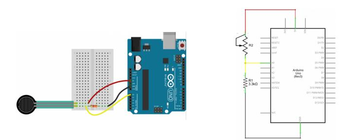
where 5v power supply from Arduino applies on the circuit. To avoid short circuit, we add an additional  $3.3k\Omega$  resistor *R1* in the circuit. Then, we measure the voltage over the *R1* with respect to the ground, and the measured value is used as input into Arduino's input port *A0*. To get the relationship between force applied on FSR and the input of *A0*, we need to first study the dynamic behavior of the FSR:
