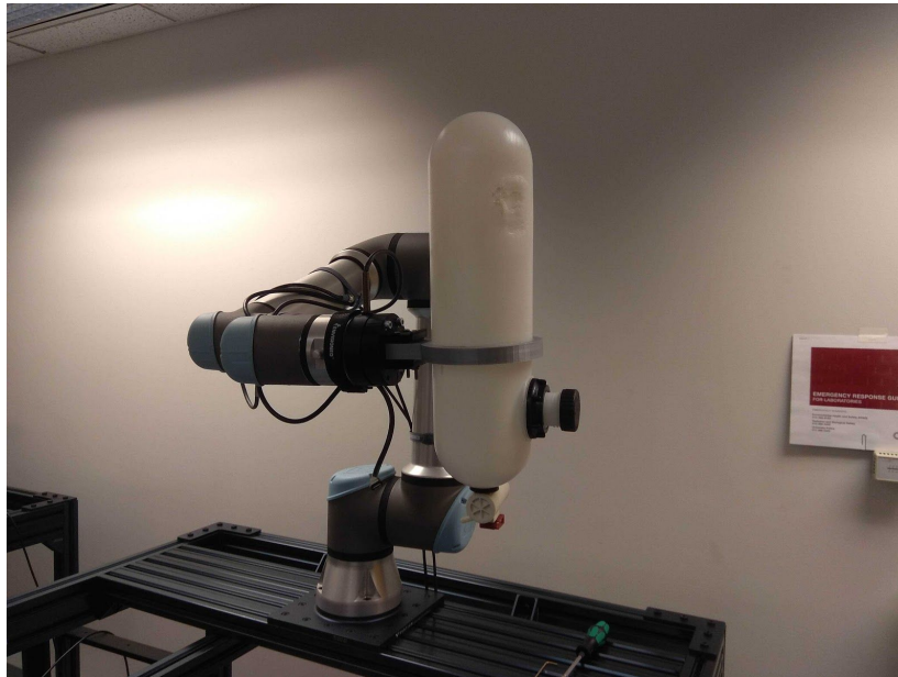
Figure 2: Extinguisher attached with UR5 arm
