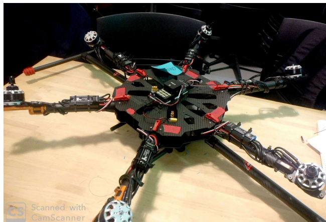
Figure 3: Newly built tilted hexacopter
