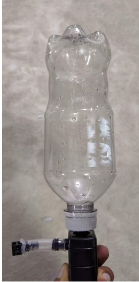
Figure 2: Extinguisher prototype with new water pump
