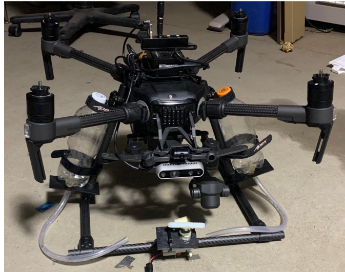
Figure 3: DJI drone with new extinguishing mechanism attached.
