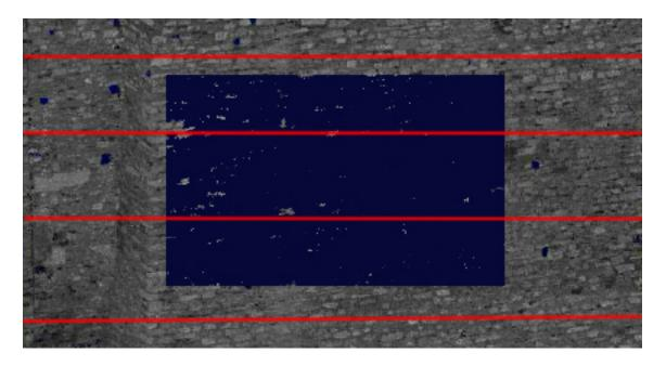
And for each horizontal scan, we apply sliding window to find the edges: for instance if the window size is 100, and we denote the pixel index is from i to i+100, we do a calculation as following:
