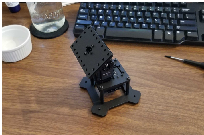
Figure 1: The PhantomX Pan/Tilt Turret, which will support the RealSense camera.
