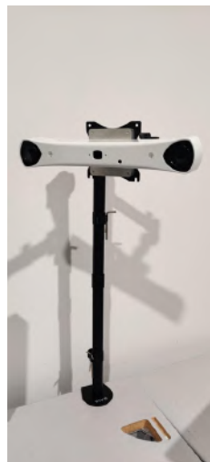
Figure 6: Camera Mounted onto a VESA Mount Using Fabricated Camera Mount Adapter
