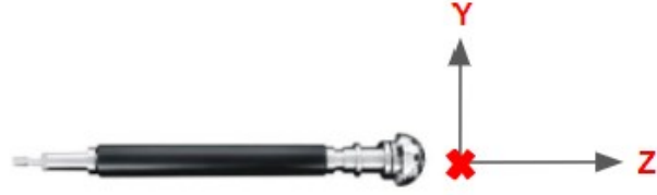
Figure 2: Coordinate Frame of the End-Effector Reamer
