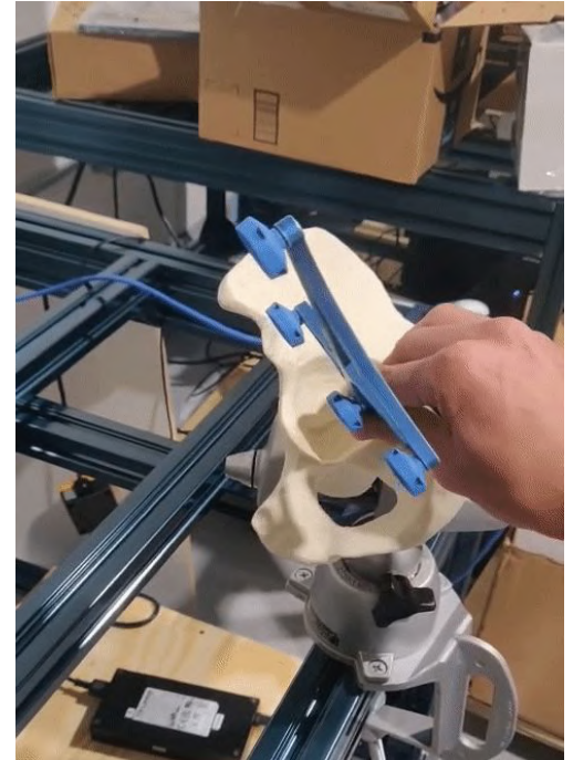
Pointcloud Collection using Registration Probe
