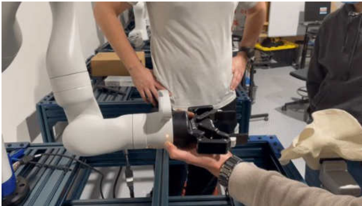
Example of Gravity Compensation in FMM
