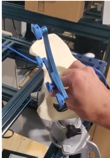
Figure 1: Pointcloud collection process from surface of acetabulum
