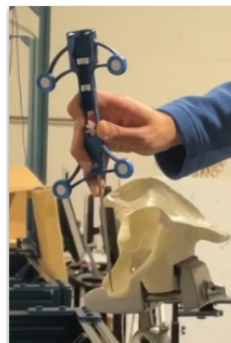
Figure 2: Registration probe used for pointcloud collection
