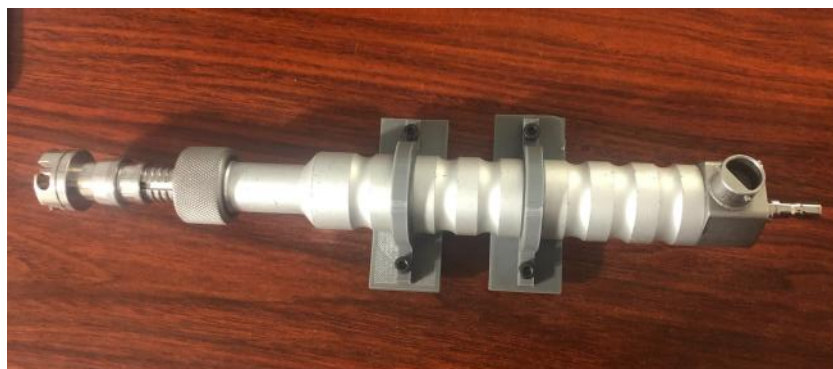
Figure 3: 3D-Printed Prototype of Reamer Handle Adapter
