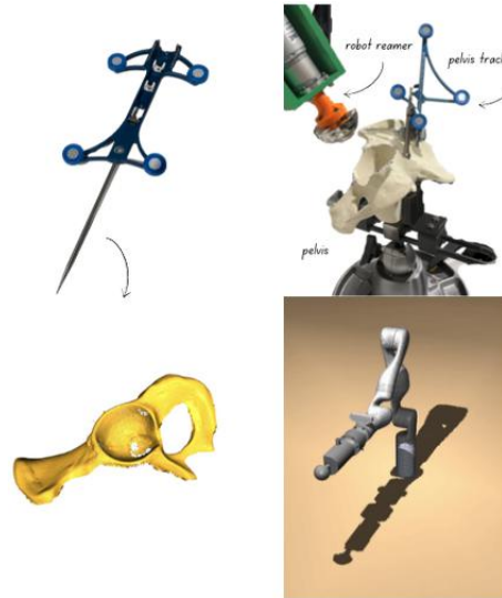
Figure 6: The various system inputs (i) Registration Probe (ii) Pelvis EE Marker (iii) Pelvis CAD model (iv) Robot Arm CAD model
