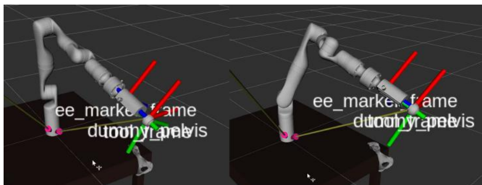
Figure 3: Implementation of Singularity Avoidance. On the left, singularity avoidance is off, so the robot moves through a singularity while tracking a dummy pelvis frame. On the right, singularity avoidance is on, so the arm reconfigures itself in its redundant space to avoid singularity while tracking the pelvis.
