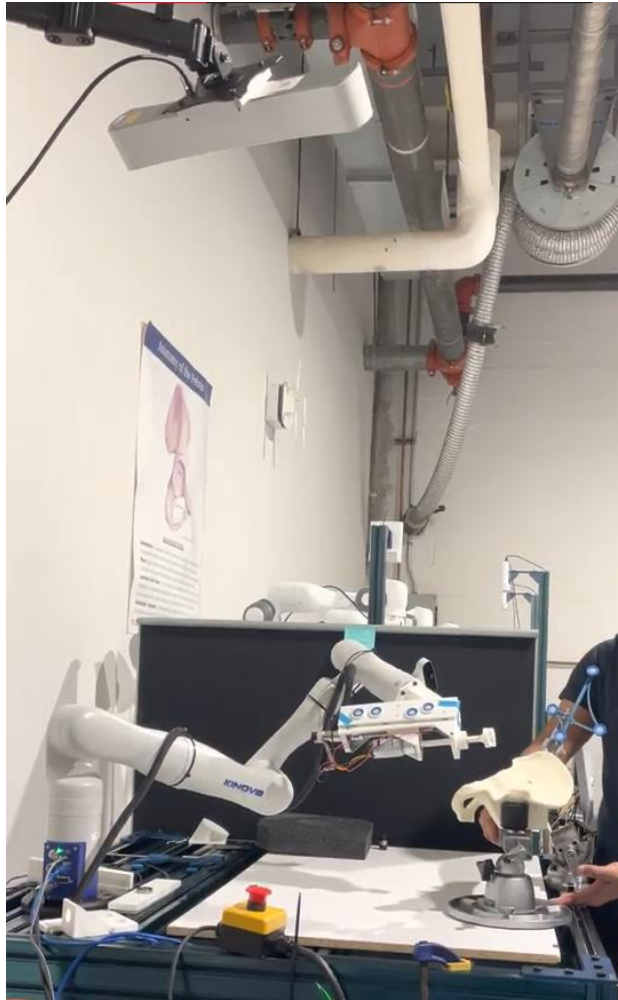
Figure 4: Task Prioritization Algorithm In Action. The arm's primary task is to track the pelvis position and orientation. With the remaining DoF, it moves the end-effector markers to align with the camera as much as possible, and moves the arm in null space to avoid singularities.
