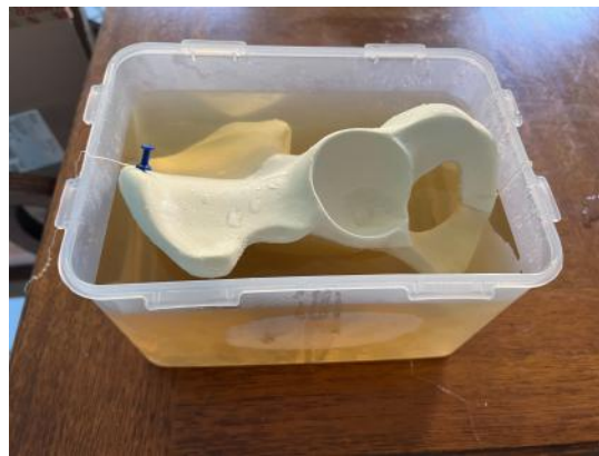
Figure 3: Ballistics gel after setting for 24 hours
