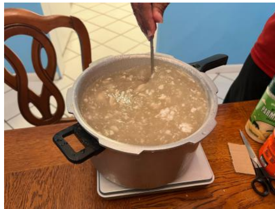
Figure 2: Ballistics gel solution before removal of lumps and setting
