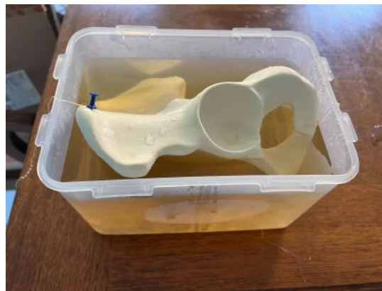
Figure 2: Pelvis model suspended in ballistics gel
