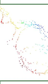
We use ICP (Iterative Closest Point) to perform registration between the **collected pelvis pointcloud** during surgery with the pre-surgical pelvis CT scan.
