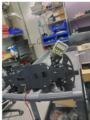
Figure 7. Steering angle mapping on RC Car
