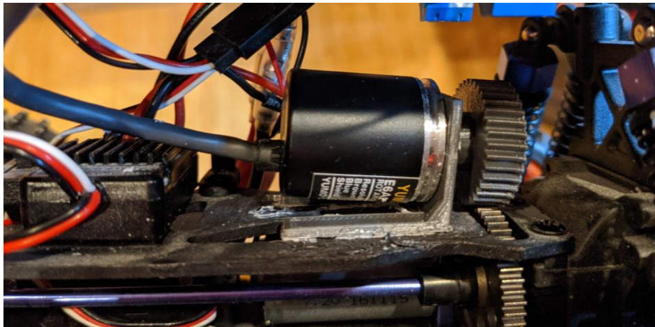
Figure 3. Encoder mount on RC Car with gear mesh
