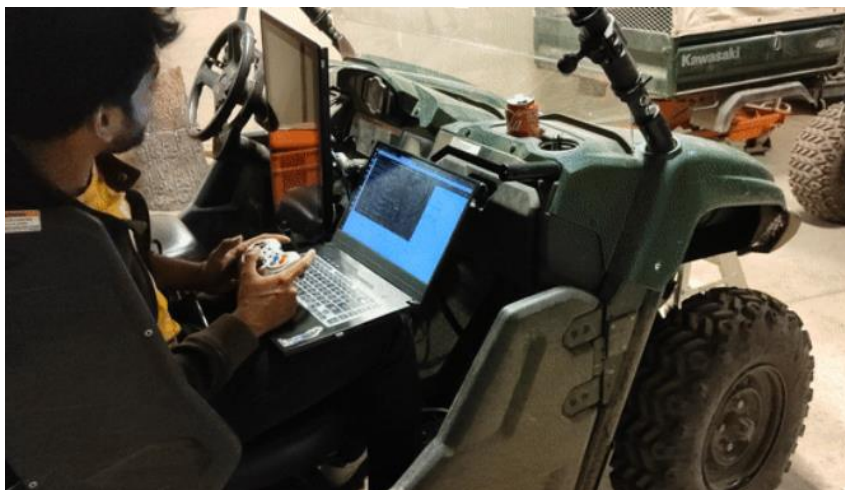
Figure 2. Drive by Wire control validation
