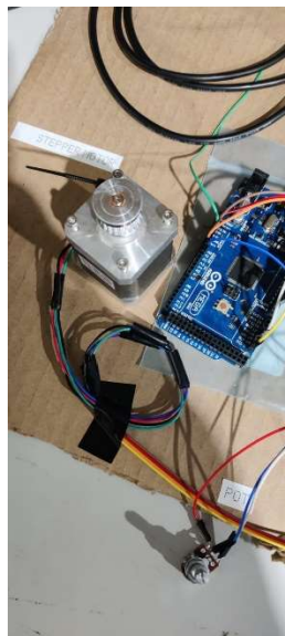
Figure 1. Stepper motor and potentiometer interfaced with Arduino Mega
