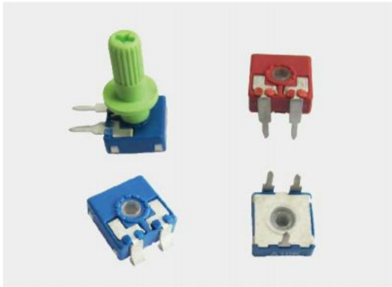
Figure 6) CA9 Trimmer Potentiometer [2]
