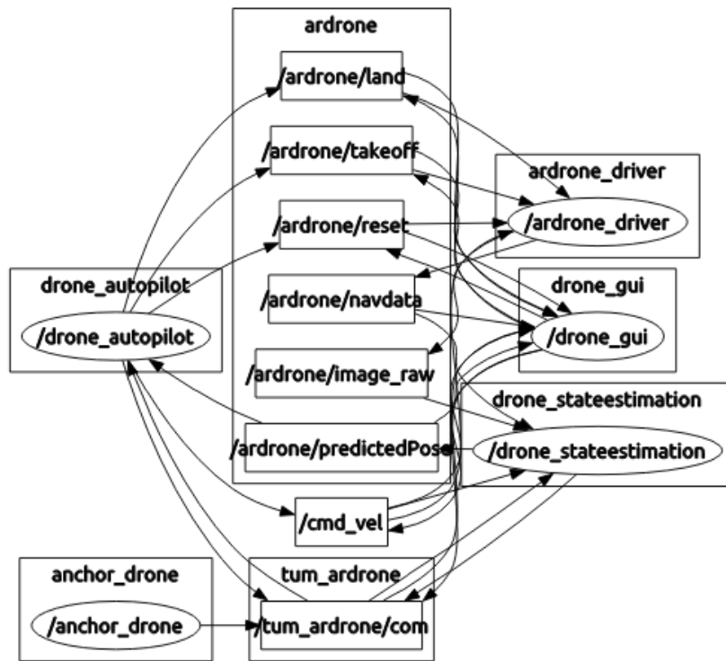
Figure 4: RQT node Graph of Tum_Ardrone with TeleOp node (anchor_drone) passing messages to the Tum_Ardrone computer
