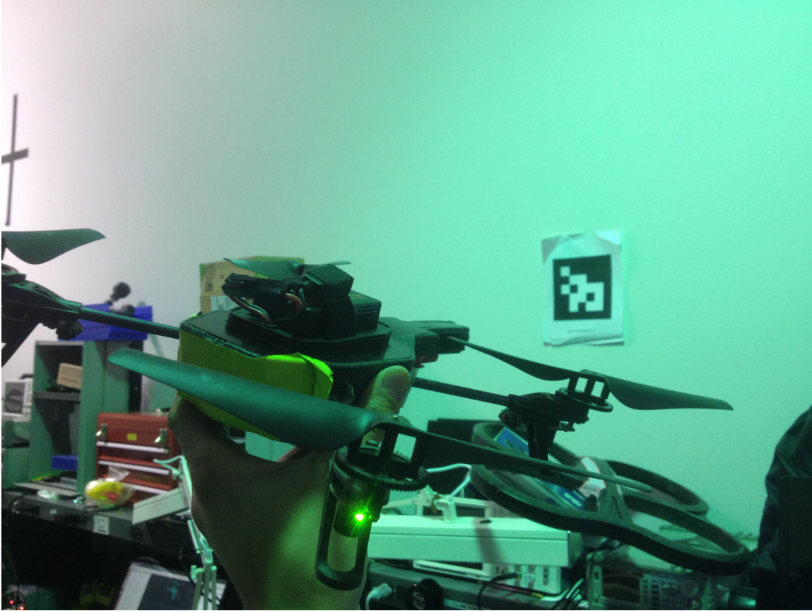
Figure 5: April Tag Testing, Drone pointed at April tag
