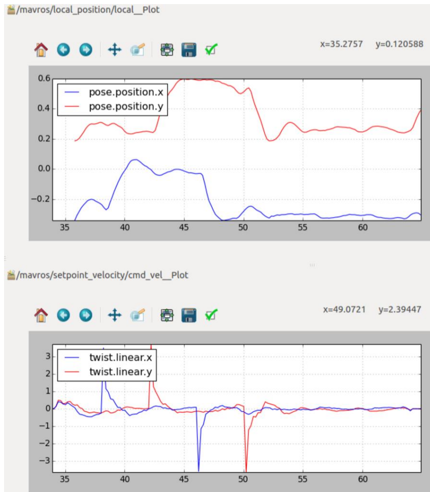
Figure 2: Square flight pattern under enhanced PD Controller
