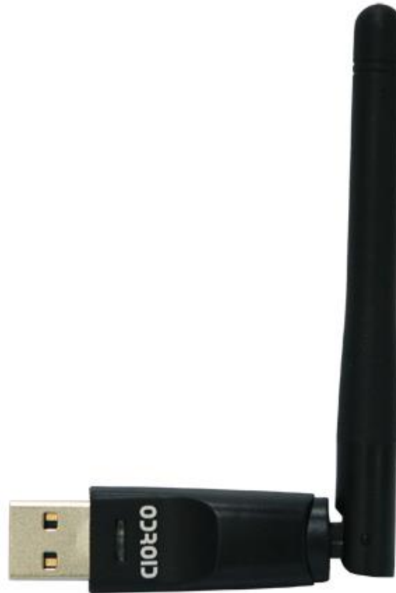
Figure 2: The Realtek RTL8188CUS-GR single-chip Wireless LAN (WLAN) USB2.0 network interface controller compatible with the 802.11n specification
