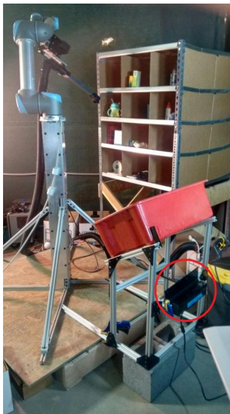
Figure 1: Image showing the setup for backup identification pipeline. The secondary Kinect-V2 (highlighted in red) facing upwards is used for this purpose
