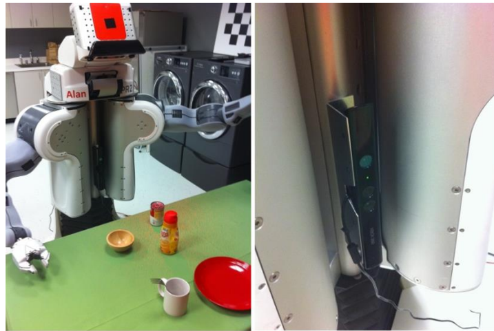
Figure 23: Possible Kinect Mounting Configuration
