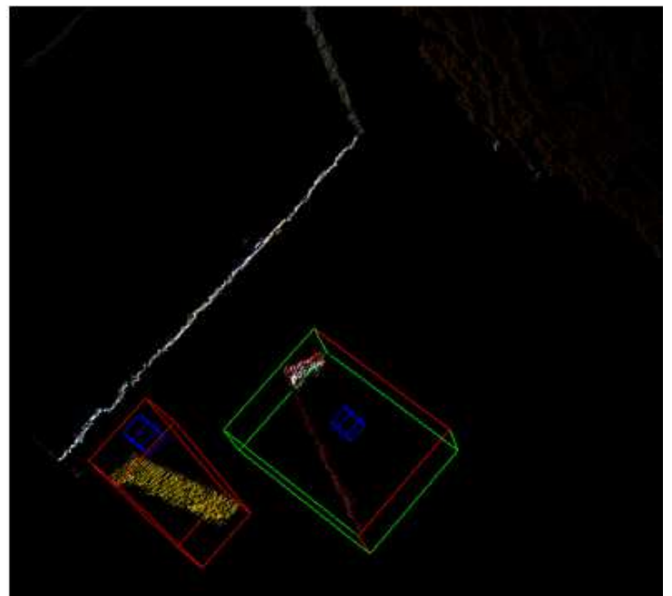
Fig 1 Representation of grasp point surrounded by the blue cube(visualization)
