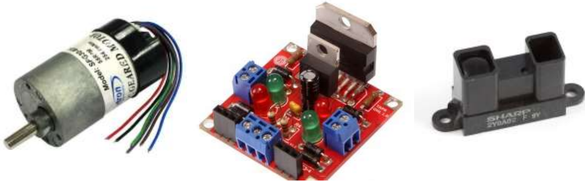
Figure 1: DC Gearmotor with Encoder, Solarbotics L298 Motor Driver, Sharp IR Range Finder
