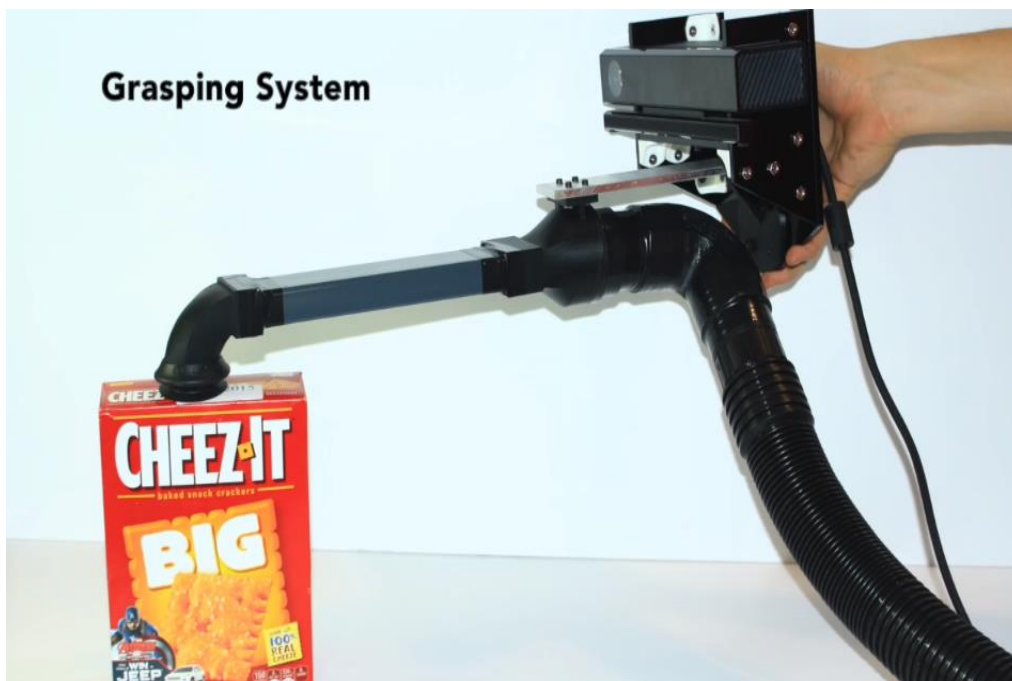
Figure 1: Image displaying the grasping subsystem with custom end-effector and Kinect2 mounted which will be attached to the UR5
