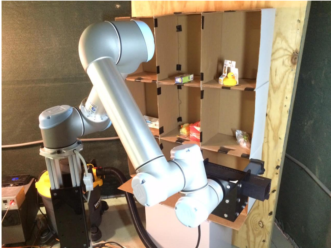
Figure 3: UR5 arm mounted on the base and 9-bin shelf visible in the background
