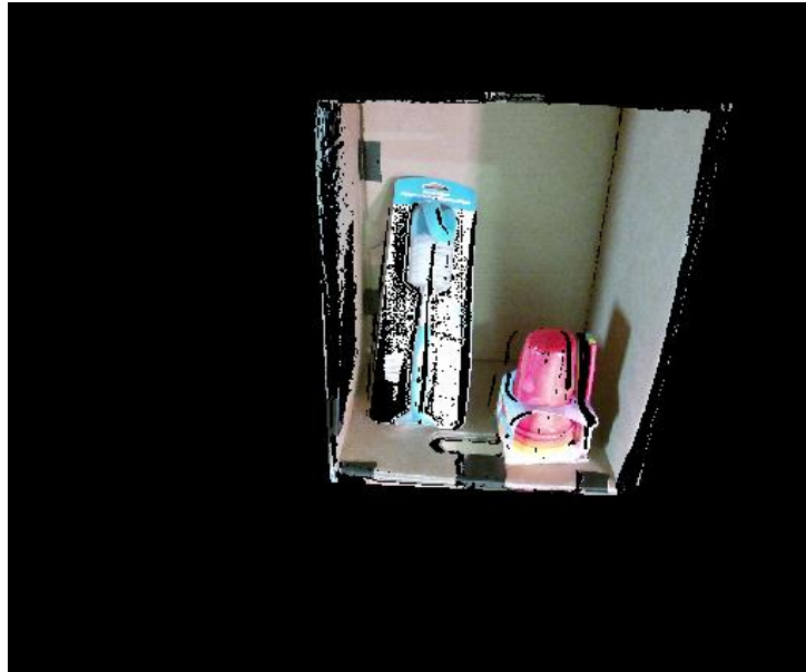
Figure 2: Image displaying the shelf scene after segmenting out the shelf of interest
