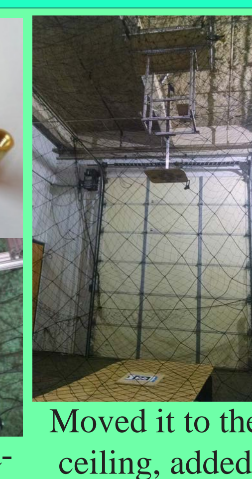
Moved it to the ceiling, added a camera so it could read an April Tag on the quadcopter
