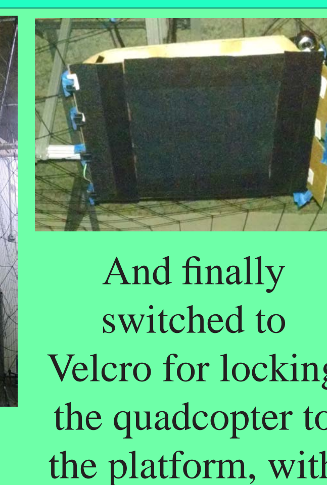
And finally switched to Velcro for locking the quadcopter to the platform, with a set of IR sensors to tell when it happened
