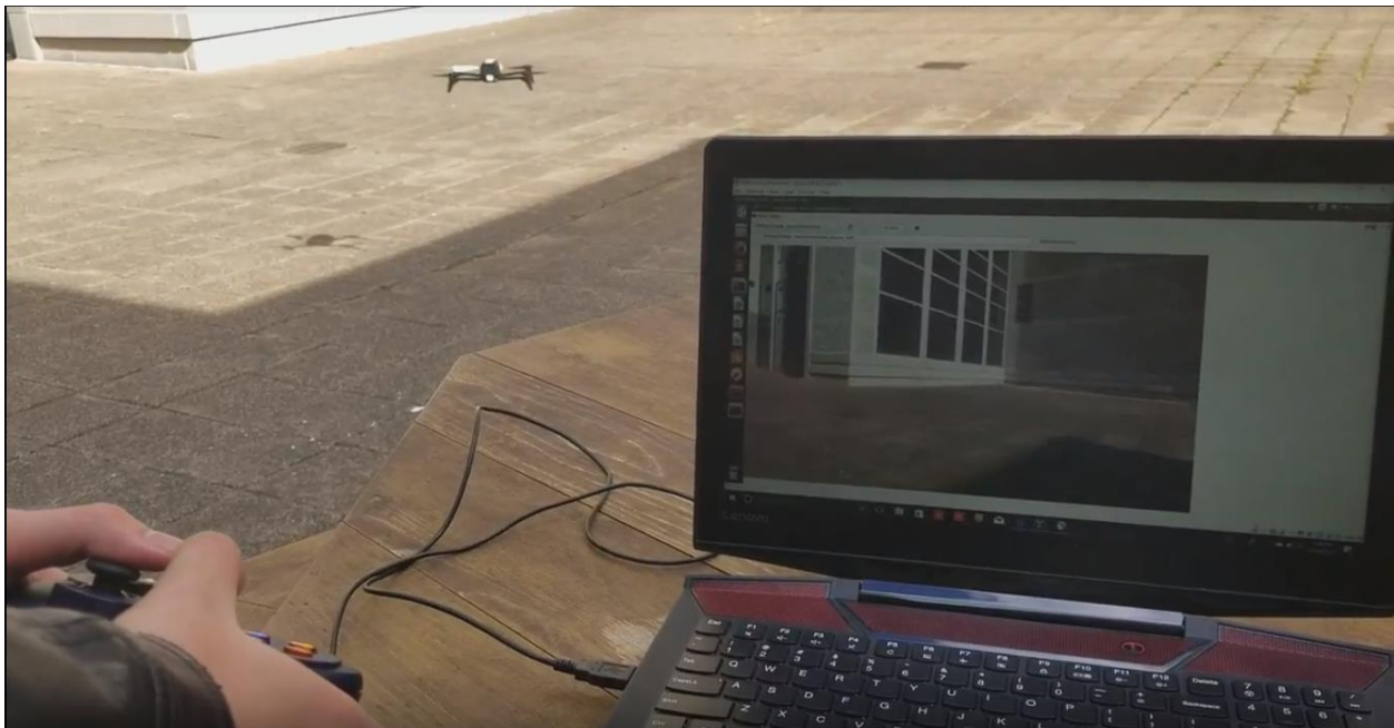
Figure 2: Drone Tele-Op using a Game Controller with ROS
